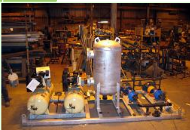
Saturator Vessel Skid under manufacturing
