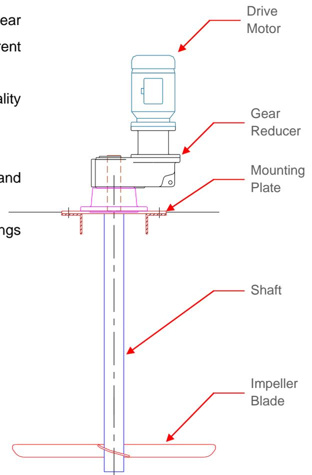
**Schematic Diagram of Flocculator**
